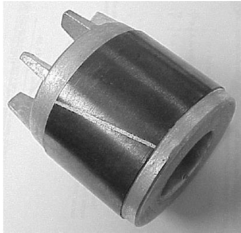
Fig. 2-4 Rotor of squirrel cage induction motor from externally
