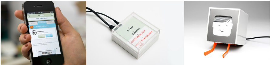
FIGURE 7-32 Commonalities across BERG's Bridge, Little Printer, and app: use of color (light green and orange accent); typeface use in app and on bridge; material and finish of white plastic across bridge and the device itself (images: BERG)
