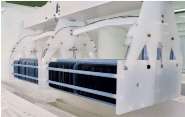
Carriers for loading wafers in the batch tool. Source: RCT solutions GmbH.
