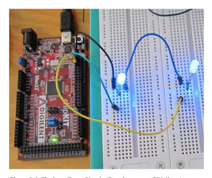
Figure 5-2. The Loop Tester Circuit. (Board courtesy of Digilent.)
