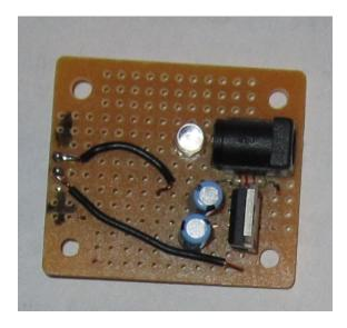
Figure B-1. A small voltage regulator circuit.
