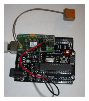
Figure 10-11. A GPS shield. (GPS shield courtesy of Libelium.)
