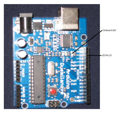
Figure 2-1. Locating pin 13 on a typical Arduino board.
