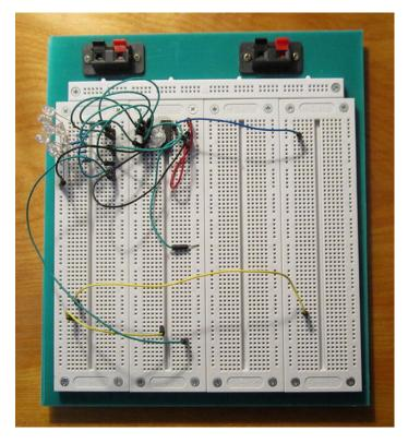
Figure 1-2. A typical breadboard.
