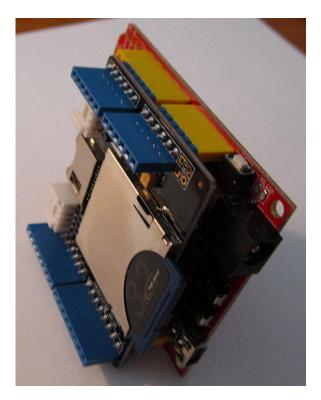
Figure 10-9. Stacked SD shield and board. (Shield and  $\mu c$  board courtesy of Seeed Studio.)
