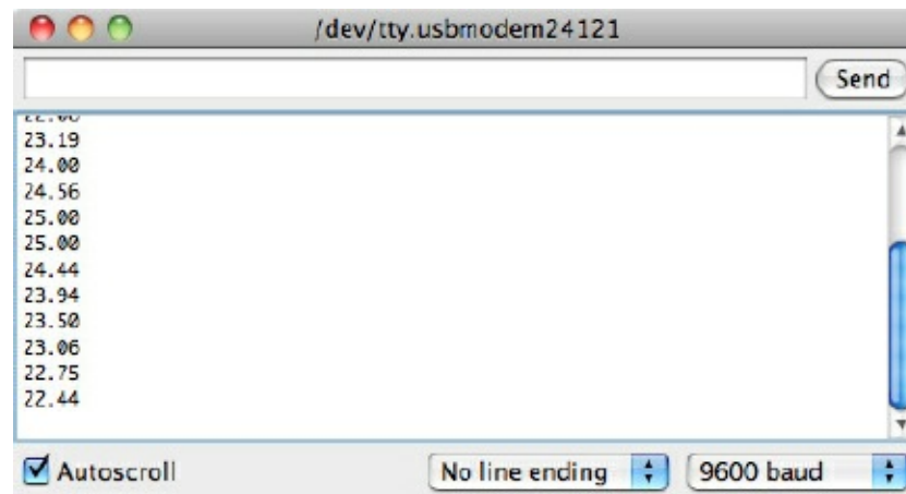
Figure 8-4 Displaying the temperature using a DS18B20
