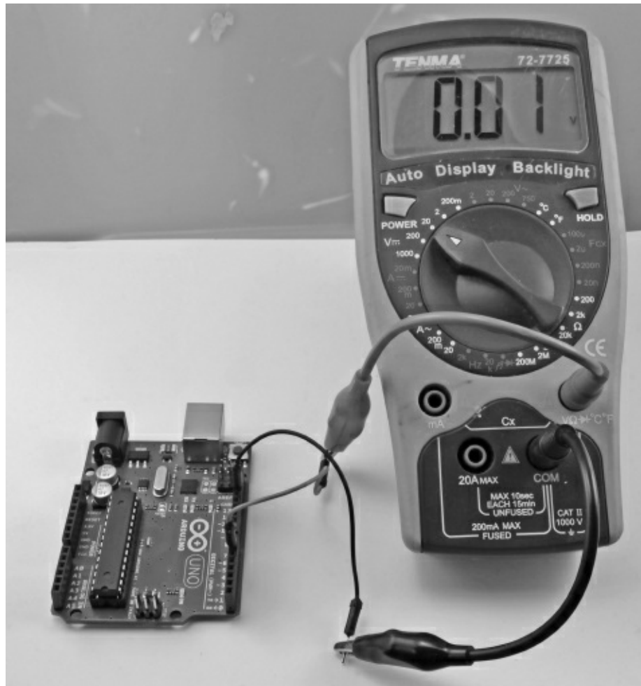
Figure 1-18 Measuring the output voltage
