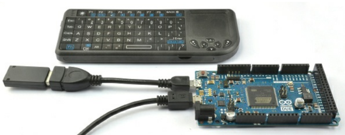
Figure 11-5 Arduino Due with a Micro USB OTG Host Cable and keyboard
