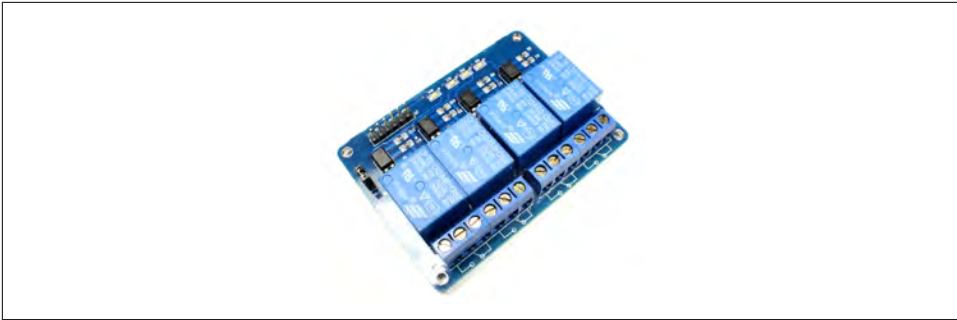
Figure 9-52. Relay module with four PCB-mounted relays
