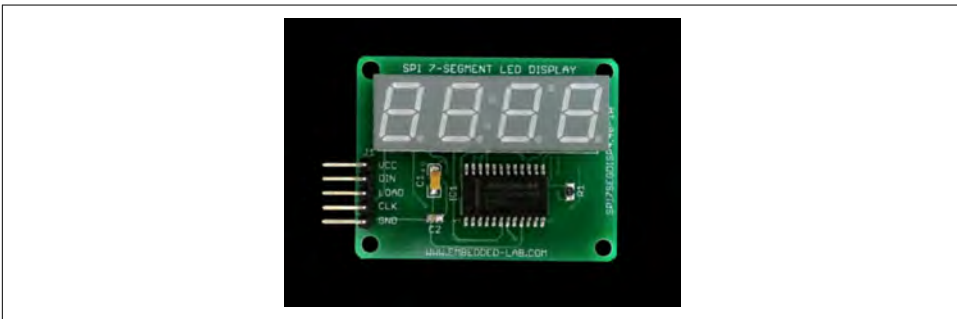
Figure 9-50. 7-segment display module with SPI interface
