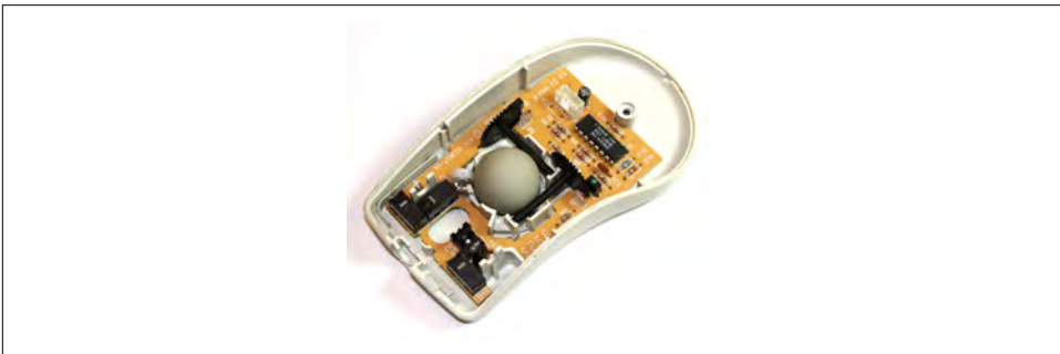
Figure 9-37. Old-style mouse with a ball and rotary encoders
