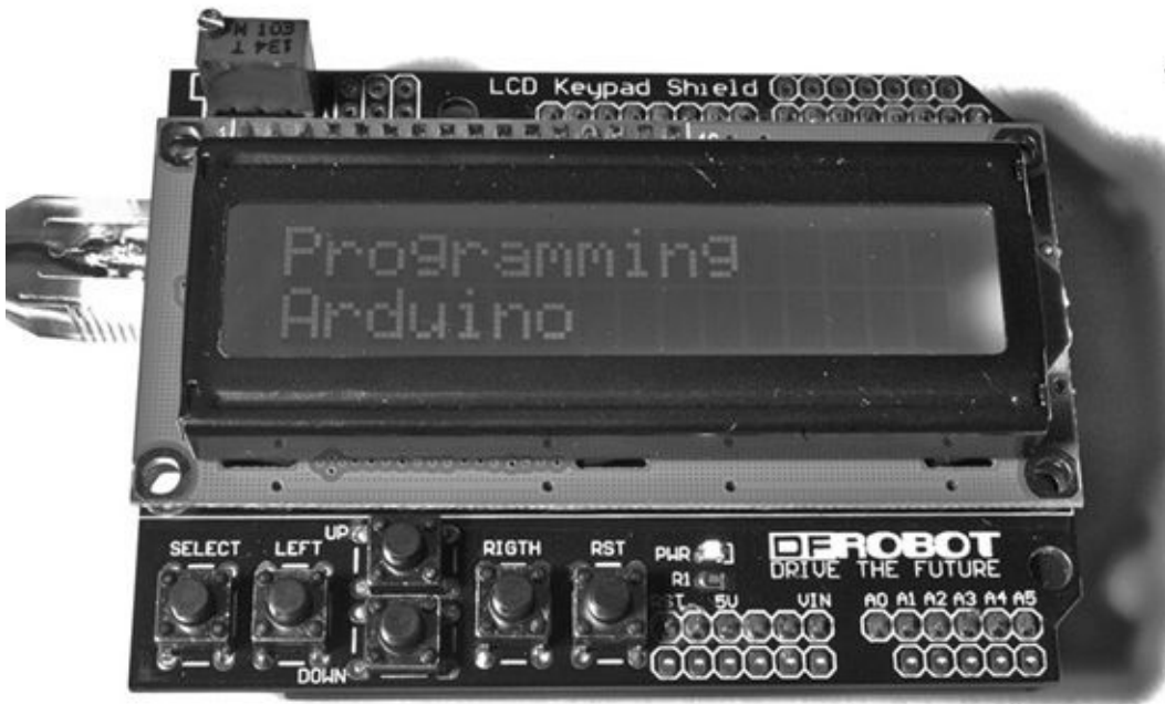
Figure 9-2 LCD shield attached to an Arduino board
