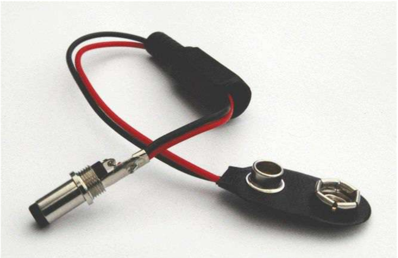
Figure 4-8 Creating a battery lead.
